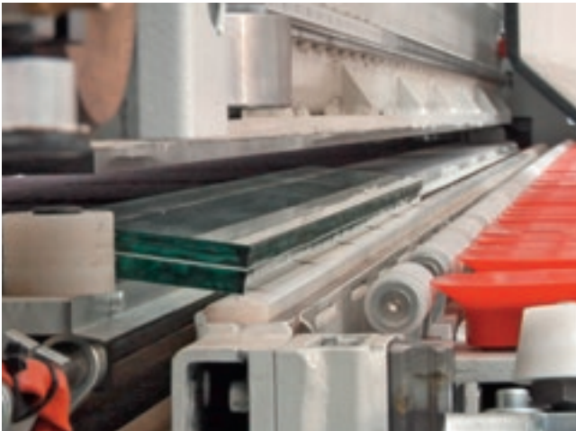
Cutting + breaking + standard removal, 60 mm.
